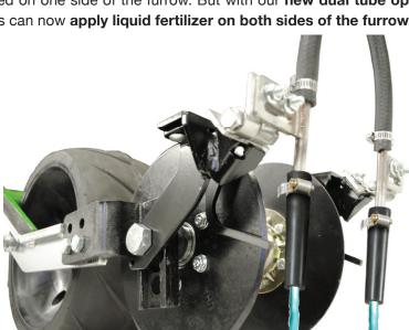
For dual side placement of nitrogen, phosphate, potash, and micro-nutrients when
