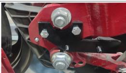
Slide the 2-1/2" x 5/16" bolts in from the outside through one of the brackets. The weldedin bolts should be in the position shown, pointing outwards and towards the back.
