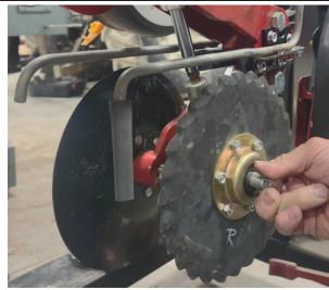
insert a 1/4" spacer bushing on the inside of the
