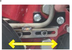
**STEP #8:** Each tube's proper location is determined by whether it is over the leading or the trailing covering disc.
