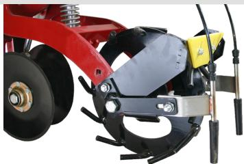
Out the Back fertilizer tubes and mounting brackets with Chicken Tracker wheel and scraper
