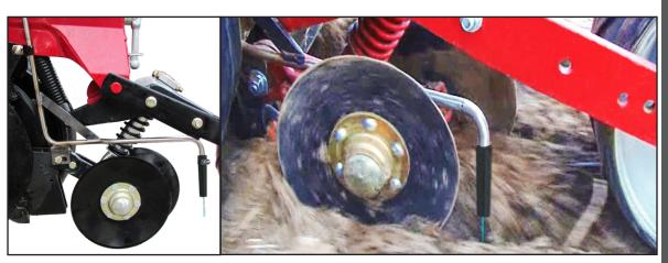
■or high pressure, screw in one of Schaffert Mfg.'s stainless steel **high pressure injector orifice** into the bottom of the tube.
