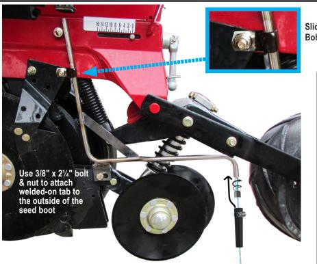
Slide tube clamp over top of tube. Bolt it to the back scraper bolt.
