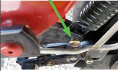
The photos below show how to tweak the stainless tube so the fertilizer will be in the furrow after the covering disc closed the seed V. Once you get into field conditions it may be necessary to bend the tube right or left or up or down to fit your needs.
