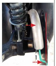
Tube needs to be bent to dotted line so that fertilizer injects directly into slice
