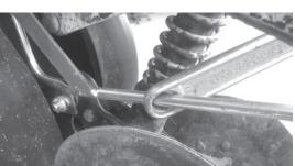
To better fit your specific planter and field conditions, you many need to tweak the fertilizer tube behind the covering disc so it squirts the fertilizer into the slice left by the covering disc.
