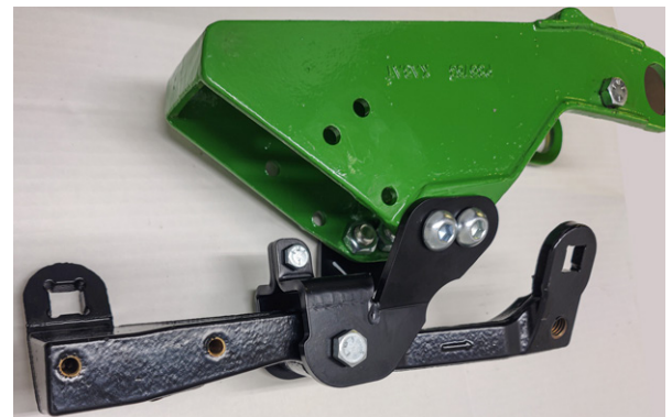
G4 arm final assembly on John Deere tail section
