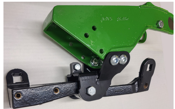
G4 arm final assembly on John Deere tail section
