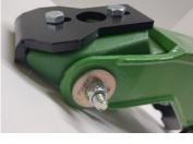
Slide stop plate in as shown in photo, with the lip toward the front and pointed down.
