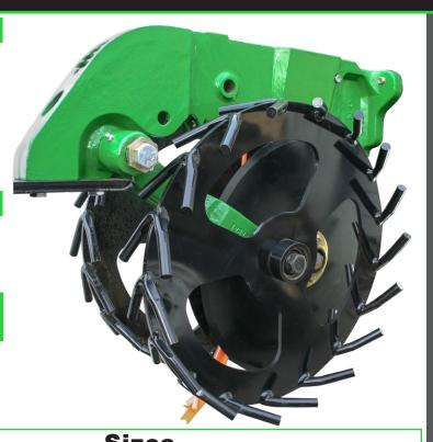
For Case IH planters and drills we have 6" and 4" Chicken 2"x12" Trackers. Both work well in no-till or minimum till fields. However. the 4" wheel has advantages over the 6" wheel, as it will work inside the 4" area being tilled by the covering discs, rather than having the 6" press wheel ride up on firm soil and not compress soil down around the seed. We also have 4" and 2" Chicken Trackers to fit John Deere, Kinze and White planters and Drills
