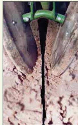
Furrow left open with rubber closing wheels
