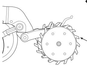
There should be **2"-2.5" distance between the cast rings,** measured directly under the lowest point of the rim.
