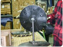
Use a butterfly wrench set to 4-5 or a torque wrench set to 100 inch-pounds to screw and tighten all six 1/4" whiz nuts on the bolts.
