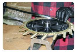
**Pull the ring away from the spot, and begin inserting the rubber insert here.** This will make it easier to get the insert in all the way around.
