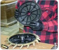
Remove the wheel from the bolt and place on flat table.
