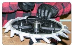
**Use a screwdriver** to help wedge the entire rubber insert in place.
