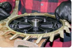
Place the ring over the rim. Most of the rings have a very slight egg-shape. **Find the place where the ring is closest to the rim.**
