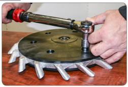
If using a torque wrench, 100 inch-pounds is enough torque.
