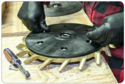
Insert all six 1/4" x 1" bolts. For Zippers, the spikes should be pointed AWAY from the boltheads.
