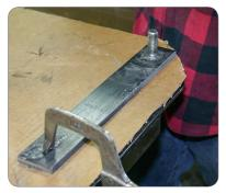
We welded a 5/8" bolt to a piece of flat iron and held it down with a clamp to make inserting the rubber insert easier.
