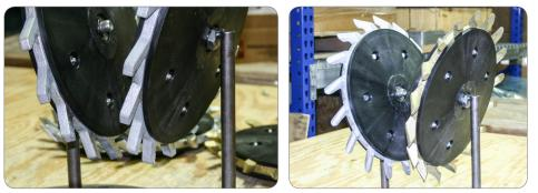
If you're standing behind the planter looking at the mounted Mohawk or Zipper wheels, the spikes should be pointed down in the back. Zipper spikes should be pointed out.
