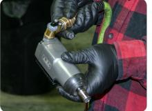
We welded a 5/8" bolt onto a stand to hold the wheel while bolting it together. We used a butterfly wrench for screwing and tightening the bolts and whiz nuts. The torque was set between 4 and 5.
