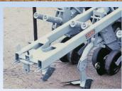
Telescoping trailer hitch provides easy hookup to fertilizer tanks. Hitches are also available for cultivators equipped with lift assist wheels.
