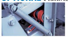
Auxiliary down pressure springs (shown in red) provide extra penetrating power in tractor wheel tracks.
