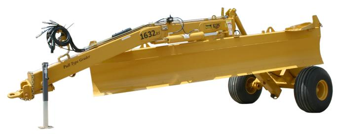
Whether you use it to grade roads, remove snow, dig irrigation ditches or clean feedlots, the Model 1632 Grader/Box Scraper is designed to move material quickly and efficiently. Productivity starts with a 16' by 32" blade with a 6" forged replaceable cutting edge for wide coverage with each pass. Transport width can be reduced to as little as 8' 4" with the blade cylinders unpinned and placed in transport position.
