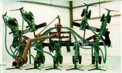
The Sukup 9400 is actually two tools in one. It can be used to cultivate and to apply liquid manure. The 9400 is the ideal tool for deep placing liquid manure. Since the 9400 causes minimal soil disturbance it places the liquid waste well under a layer of soil and residue, where it is unable to ooze back out over the top surface. It is placed, and remains, in the root zone, where it is most valuable to the plants.
