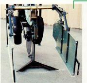
Optional Open-Top Shields are independently mounted to allow better residue flow and to provide maximum protection for crops of all sizes. The galvanized construction and bushings at the wear points ensure optimum performance and long life. Spray shoes for use in cotton are standard.
