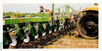
*Heavy-duty, massive double toolbar* provides maximum strength and support for 12-row wide through 16-row narrow cultivators.
