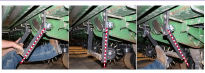
Its torsion axle allows the Stalk Destroyer full back-and-forth flexibility, stomping down all stalks upon contact without getting hung up in ditches or over terraces.
