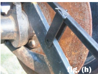
Fig. (h,i,j) mount on the unit where the press wheel was, sliding it down into place. Fig. (k) tighten the nut down against the down pressure arm.
