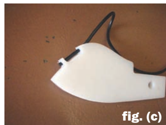
Fig. (b,c,d) displays the threading of the hose through the Fin.
