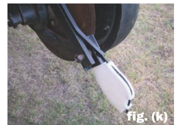
Fig. (h,i,j) mount on the unit where the press wheel was, sliding it down into place. Fig. (k) tighten the nut down against the down pressure arm.
