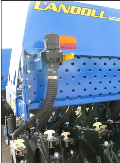
fill hose out the back of drill
