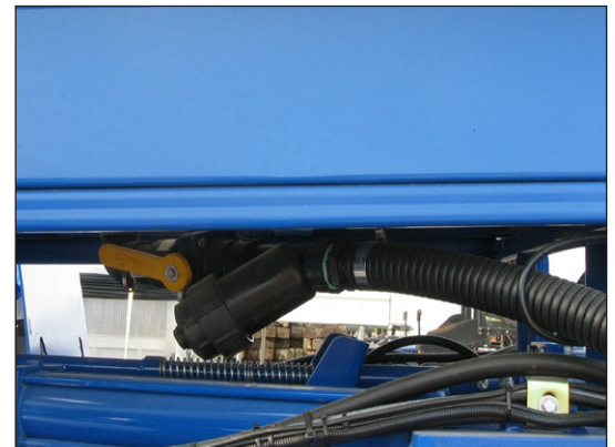
bottom of tank and filter system
