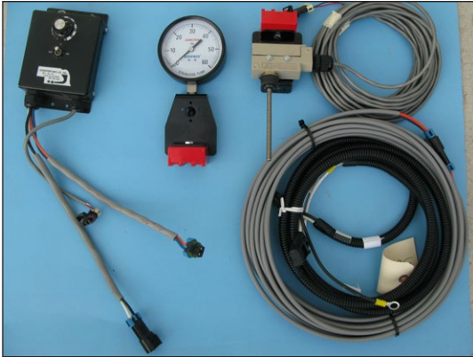
controller (left); Run Hold (upper right); power cords (lower right—black one goes to battery and grey ones go to pumps on drill); pressure gauge with mag mount (upper center)
