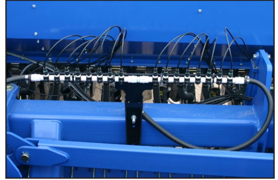
manifold on one section
