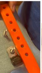
Place the tube clamp over the bolt with the flat edge towards the seed tube and the round coated edge at the bottom.
