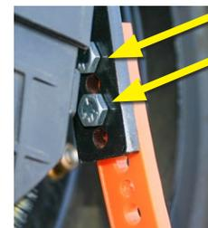
bolts go through 1<sup>st</sup> (top) and 3<sup>rd</sup> hole on mounting bracket
