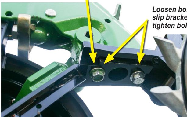
Loosen bolts, slip bracket in, tighten bolts
