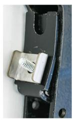
**#5:** Place the Rebounder over the bolt. You may need to **drill out the hole a little bit** in order for it to easily slide on.
