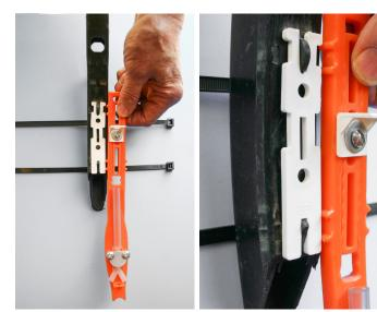
Where the Rebounder attaches on, hold in place with tie straps. Tie straps fit inside each of the two sets of notches on the outsides of the Rebounder.
