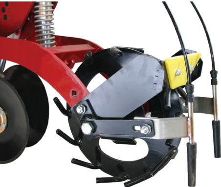
Tubes out the back with Chicken Tracker & scraper
