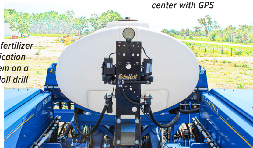
Dosatron & GX2 double pump distribution center with GPS
