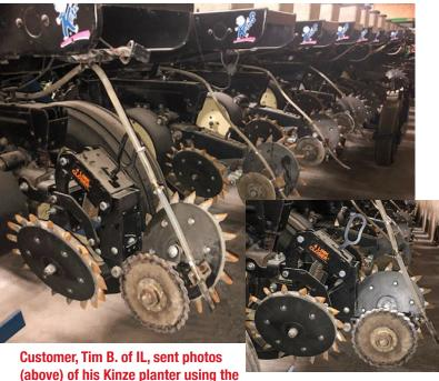
4 link closing system on one row in comparison with the factory set-up on the rest of the rows. You can clearly see the improvments made that Tim attributed to not having to run as heavy a down pressure on this row, which meant there was far less sinking and compacting of the soil with this row leading to better emergence.
