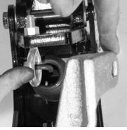
Push chrome bushing through G2 arm & slide G2 arm up into bottom of G2 mounting ears. Slide in 1/2" x 3 1/4" bolt though the ears and G2 and tighten it down.
