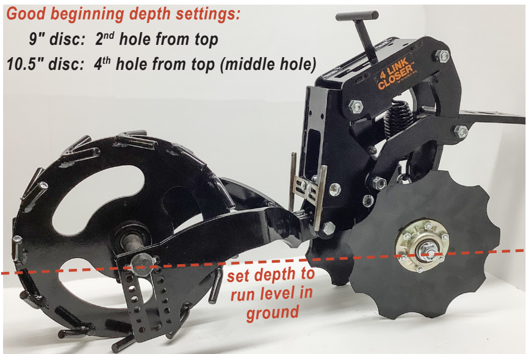
Y-CAM final assembly on 4-Link Closer shown with 6" Chicken Tracker wheel and 10" notched discs
