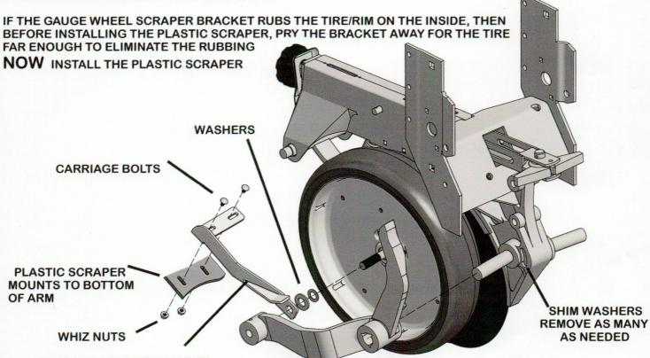
SCRAPER BRACKET MOUNTS TO GAUGE ARM
