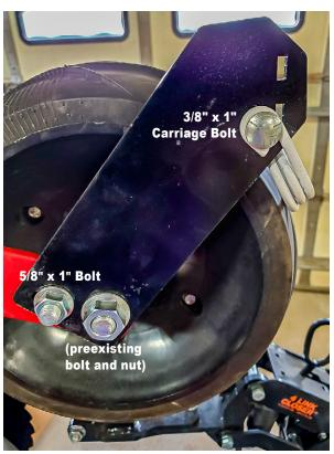
\*This scraper was designed to mount on the left hand side of the planter row unit when facing back of unit looking forward.
