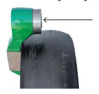
We weld our gauge wheel scraper mount to the bracket holding the u-bolt that clamps to the milled area of the arm.
