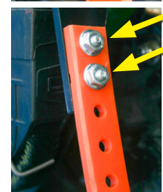
bolts go through top 2 holes on Rebounder
