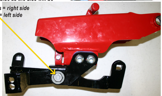
G2 arm final assembly on Horsch tail section
