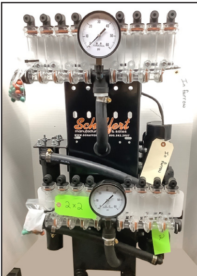
GX2 pump system with manifolds for both in-furrow and 2x2 fertilizer application
