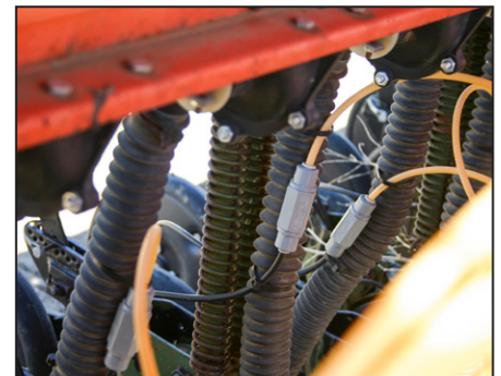
Check valve and hoses on Tye
