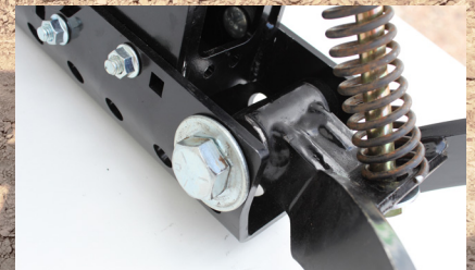
spring bracket holds spring with 1/2" washer & 1/2" lock nut
