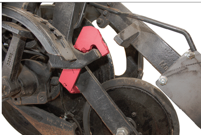
upper stop keeps the closing wheel from hitting the press wheel
