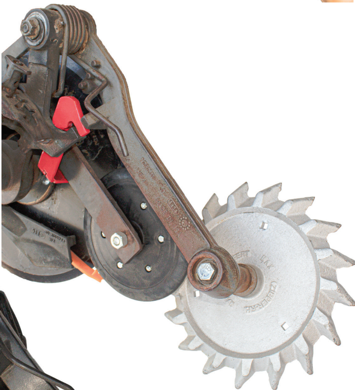
lower stop keeps the press wheel from hitting the Rebounder
